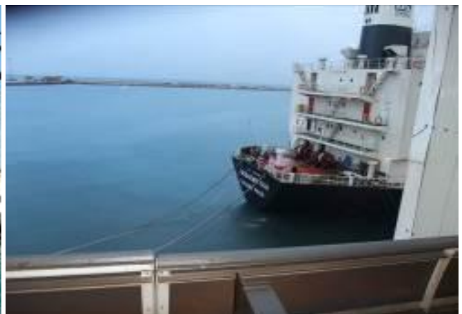
Photo 4 shows excessive slack in lines.
