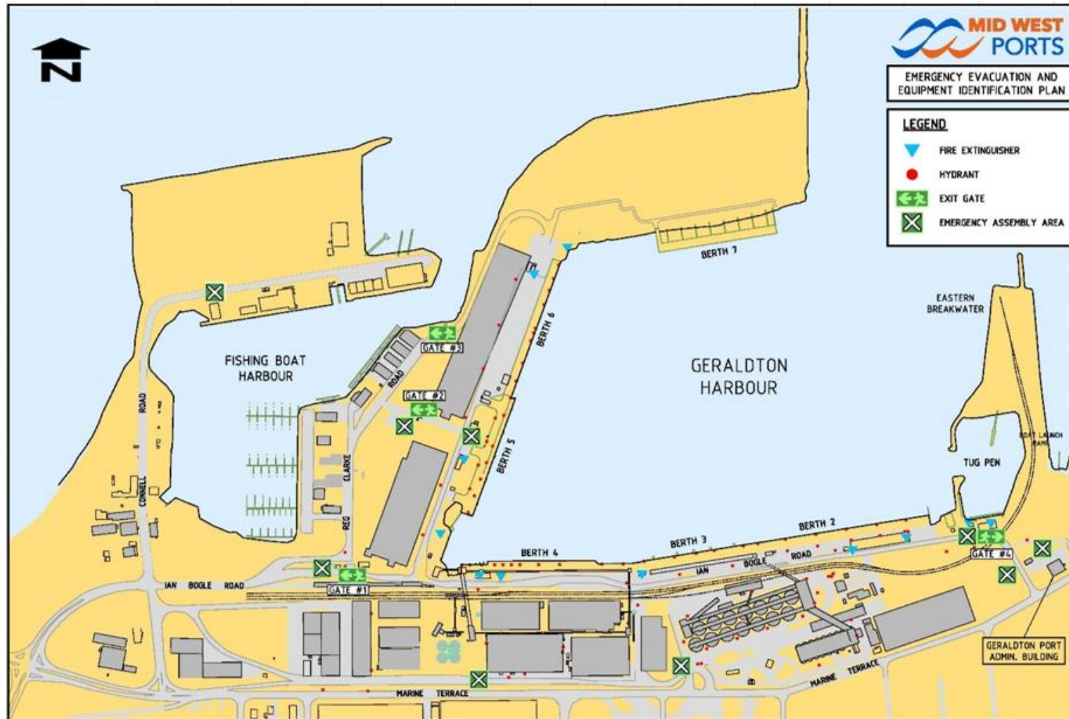
Figure 1 – MWP Emergency Equipment and Evacuation / Assembly Areas
